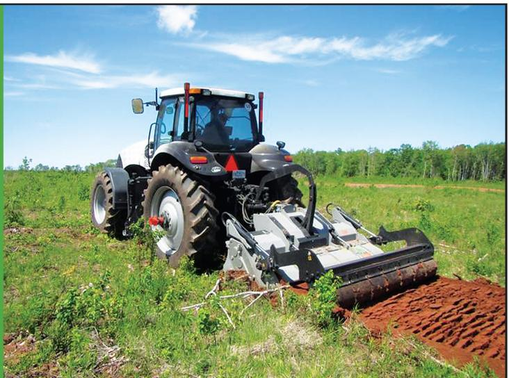
The SFM is a forestry tiller and wood mulcher capable of grinding small standing trees, large stumps and roots and immediately tilling the mulch into the soil. This innovative attachment has a working depth of 12 inches. The use of the SFM for agriculture has a significant advantage compared to the old methods of burning and burying.
